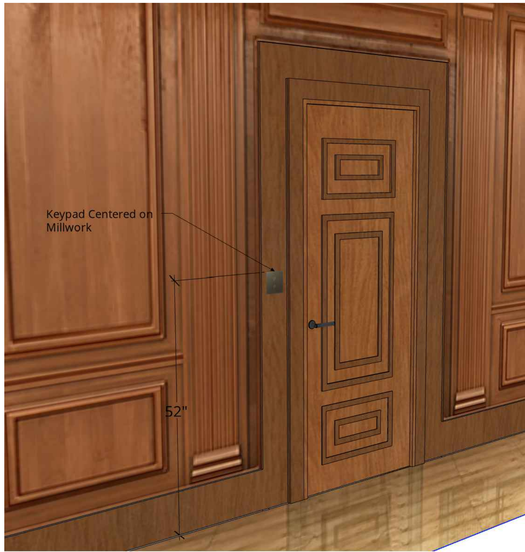
DETAIL 01 Lighting Keypad Height and Location
